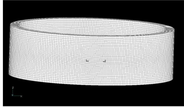
Figure 6. 3-D FEM model of static part to landing gear with semi-elliptic surface crack
