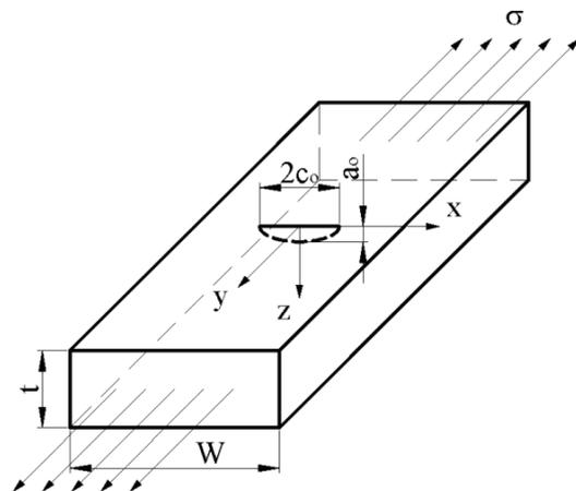
Figure 1. part one - Model 3-D solid with surface semi-elliptic crack
