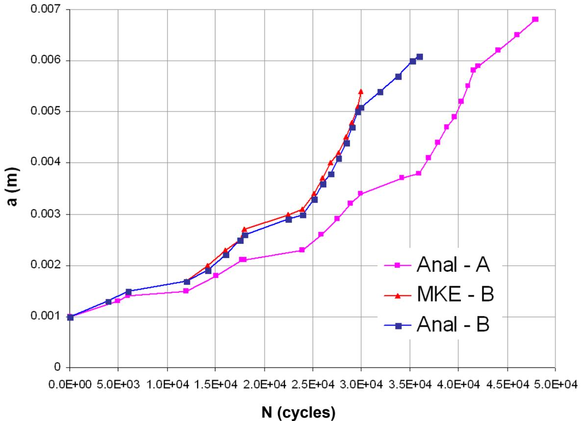
Figure 2. Results of the crack growth analysis under load spectra
