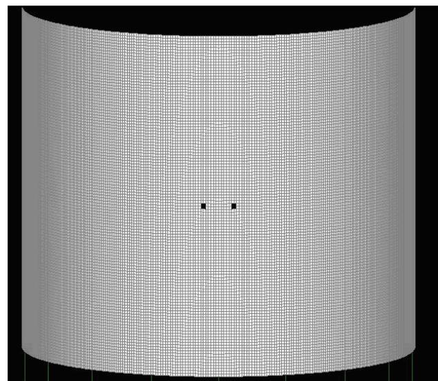
Figure 9. 2-D FEM model to static part with crack through the thickness
