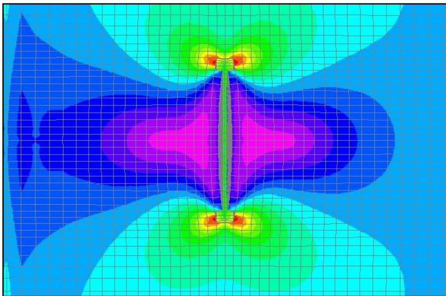
Figure 7. Detail of stress distributions around surface crack to static part of nose landing gear
