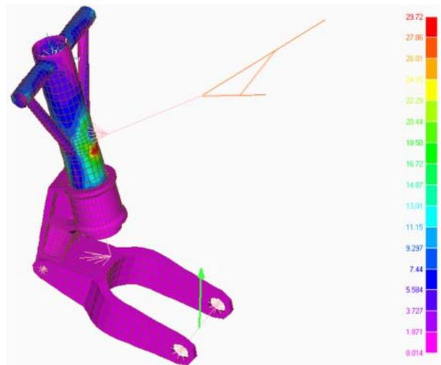
Figure 4. Finite element model of light aircraft nose landing gear
