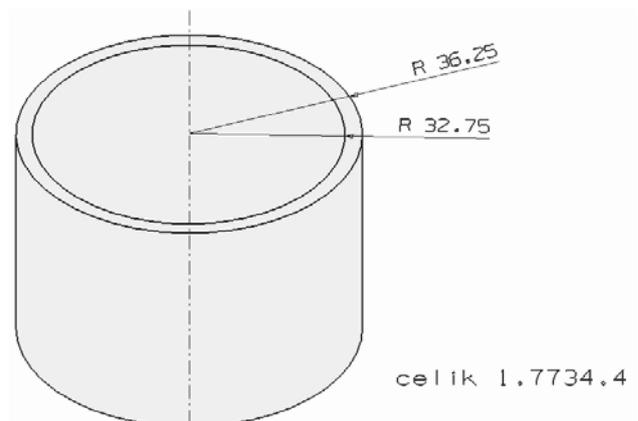
Figure 5.a. Geometry of static part under tension load ( $\sigma=10 \text{ daN/mm}^2$ )
