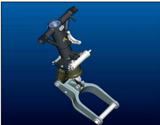
Figure 3. Structural model to nose landing gear of light training aircraft
