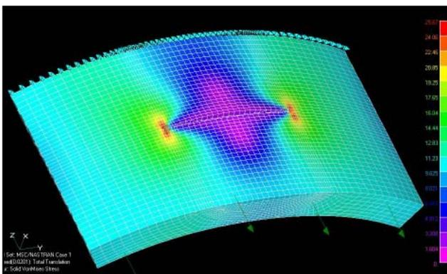
Figure 8. Detail of the stress distributions to zone semi-elliptic surface crack to static part of nose landing gear ( $a/c=0.4$ )
