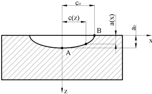
Figure 1. part two - Model 3-D solid with surface semi-elliptic crack
