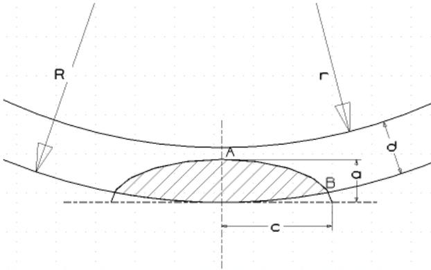
Figure 5.b. shape of semi-elliptic surface crack
